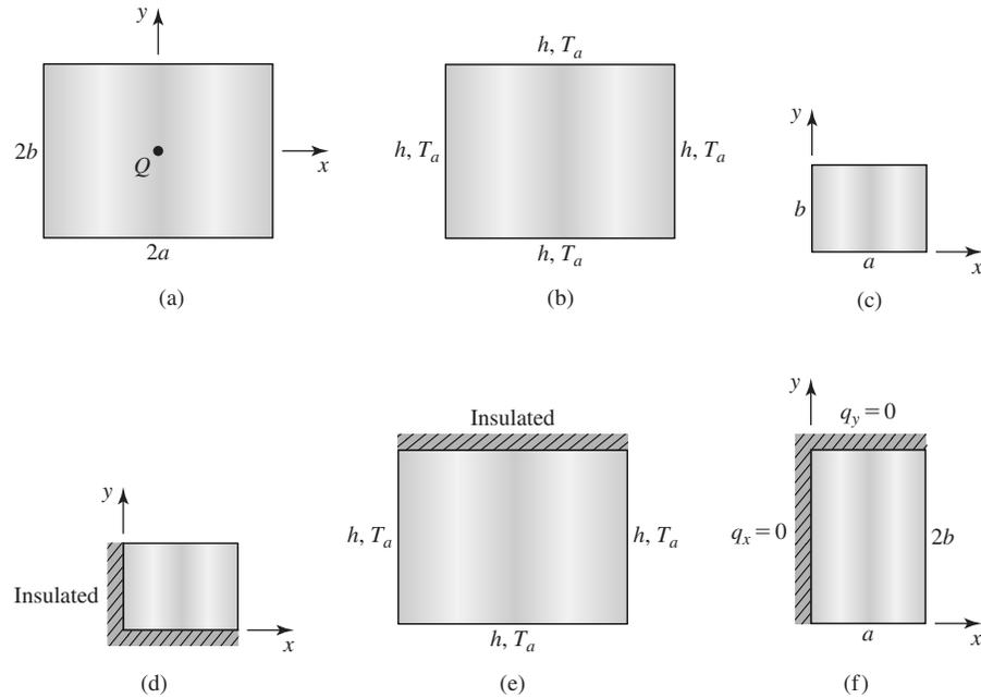
**Figure 7.12** Illustrations of symmetry dictated by boundary conditions.
