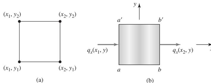
**Figure 7.7** Illustration of boundary heat flux in  $x$  direction.
