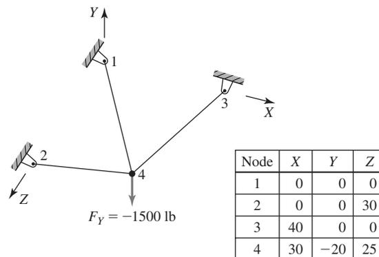
Figure P3.26 Coordinates given in inches. For each element  $E = 10 \times 10^6$  psi,  $A = 1.5$  in.<sup>2</sup>.
